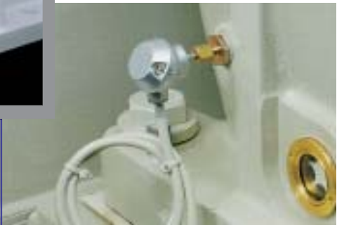
Pt-100 bearing temperature detector and oil sight-glass
