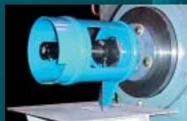
Speed measurement unit including absolute encoder and pulse tachometer
