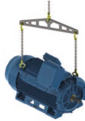
Figure 7 - Lifting with vertical chains.
